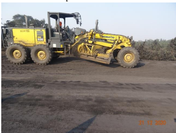
Photo: Photo of grader/scrapper used for leveling, Photo: Photo of catch drain around OB dump
