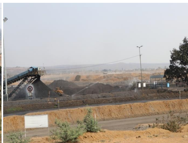
Photo: Photos of rain gun for suppression of dust near a crusher.
