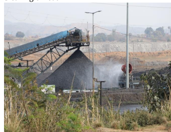
Photo: Photos of rain gun for suppression of dust near a crusher.
